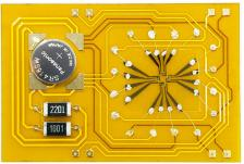
Figure 2 Portable ECG sensors based on organic monolayer OFETs
