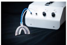
Photo 2: Prototype of mouth guard device with micro-scale mist injection function
